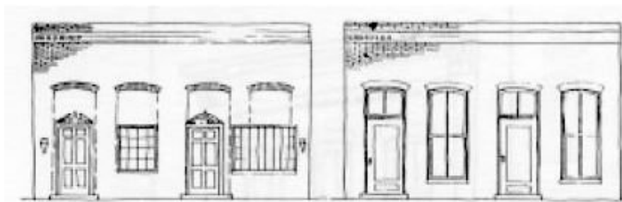
Figure 90: Added or changed doorways severely alter a building's appearance
